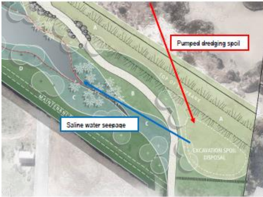
Figure 9: Proposed site for dewatering and disposal of spoil.
