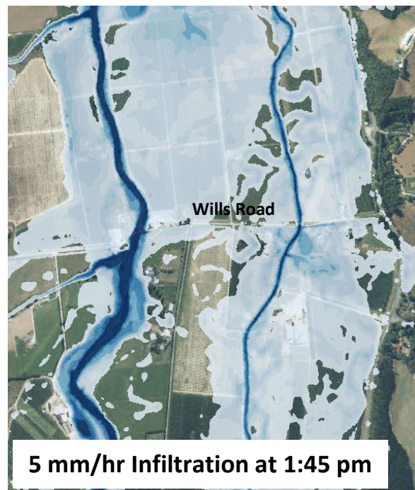
Figure 14: Aerial photograph showing Moutere River flood extent and modelled flood extent assuming 5 mm/hr infiltration in the vicinity of Wills Road looking downstream during flood event on 9 April 1976
