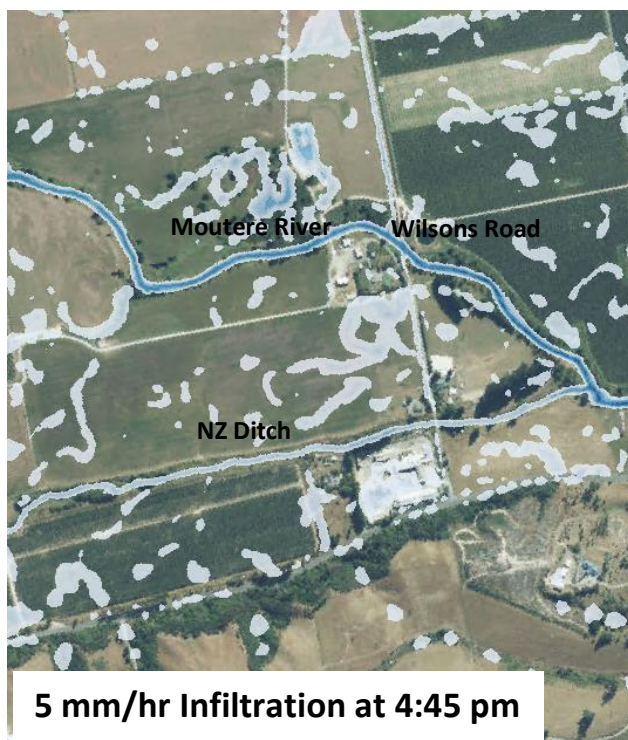
Figure 13: Aerial photograph showing Moutere River flood extent and modelled flood extent assuming 5 mm/hr infiltration near the sawmill at Wilson's Road during flood event on 9 April 1976
