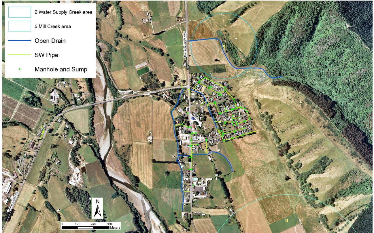
Figure 8 – Stormwater network in the Tapawera township.
