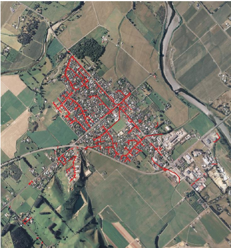
Figure 3.4. Brightwater pipe network included in the model
