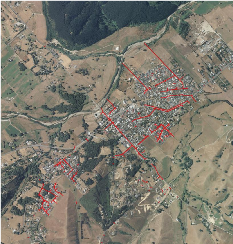
Figure 3.3. Wakefield pipe network included in the model
