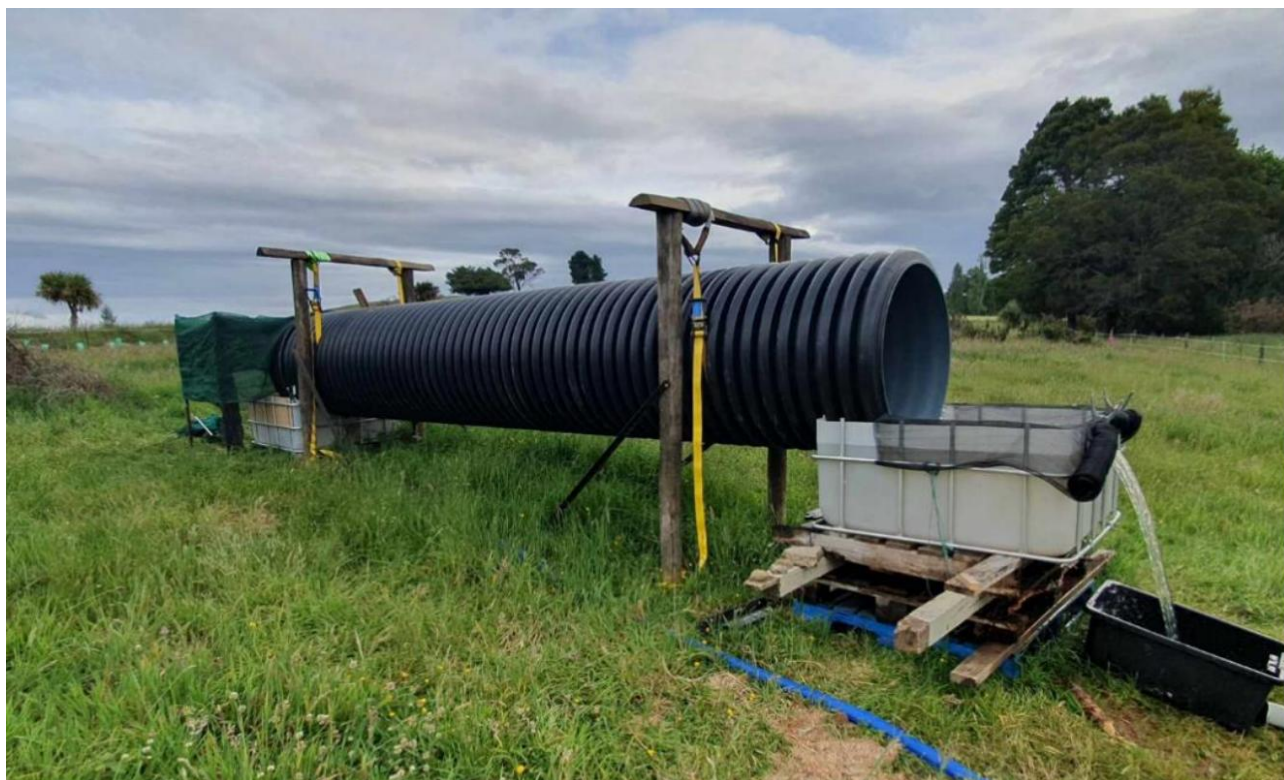
Figure 4. Experimental model culvert to test efficacy of flexible weir baffles for īnanga passage.
