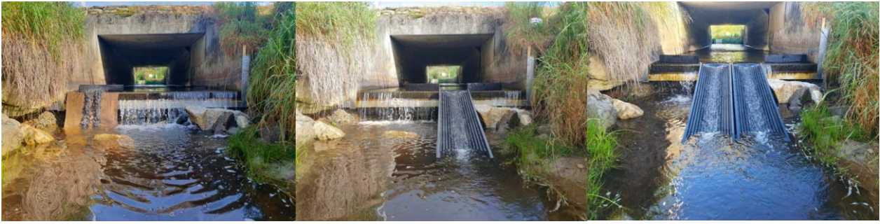
Figure 5. Three remediation treatments tested in sequential rotation at Dominion Stream, from left to right: flexible ramp and rope combination, single floating ramp, and twin floating ramp.
