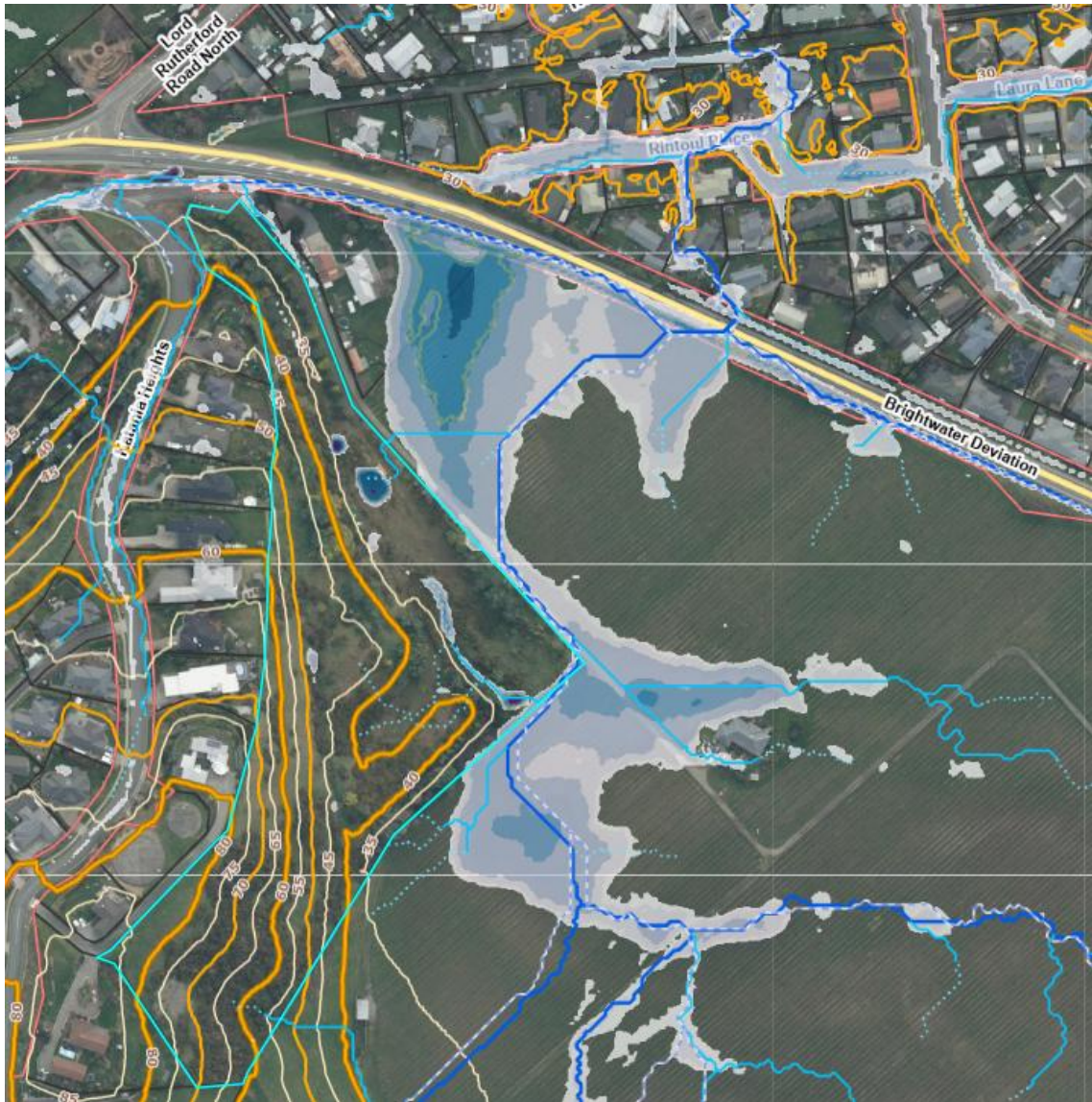
Figure 19 T-104a and b and downstream network showing existing OLFP and 1% AEP flooding
